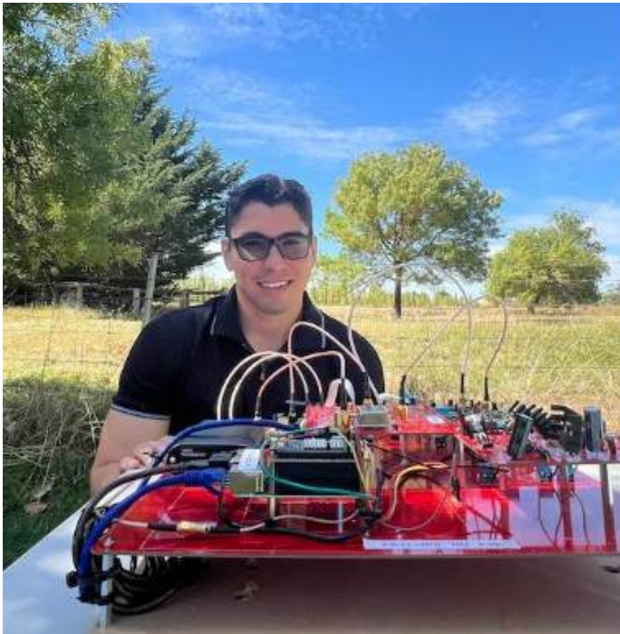
Dr Douglas Gomes working on the new device that can detect a broken conductor.
